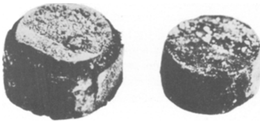
Figure 6 Macroview of the hot corroded 0.17C/0.02B (left) and 0.03C/0.2B (right) ZHS6-K alloys.
